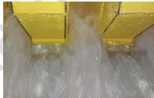
Fig. 5. Flow interference beneath the inlet keys in the sloped rectangular PKW.
