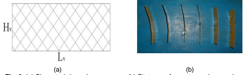
Fig. 3. (a) Characteristics submerge vane; (b) Six types of curvature submerged vanes.
